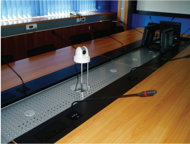
Fig. 3: Detail of rotating camera and microphone in the audio-visual lecture room
